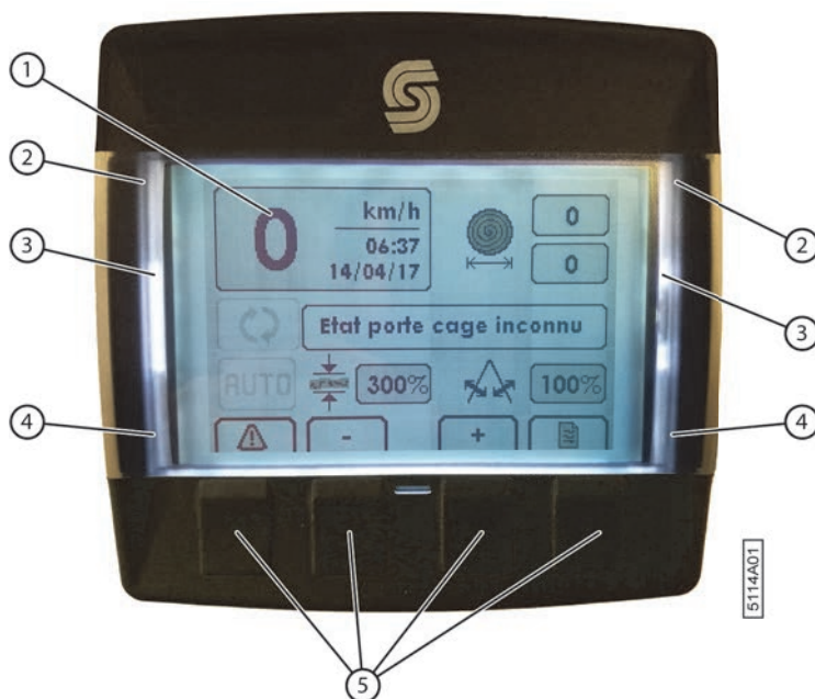
Fig. 14: The control screen
