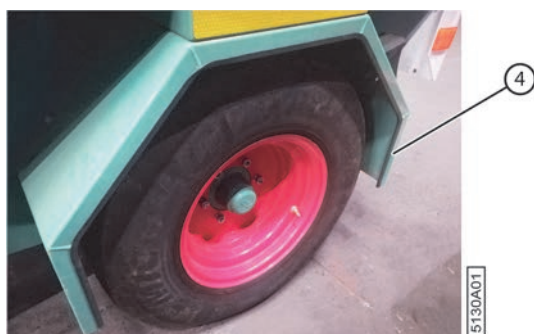
Fig. 34: Detailed view of protective panel for the edge of the mudguard
