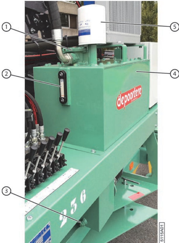
Fig. 15: The hydraulic tank
