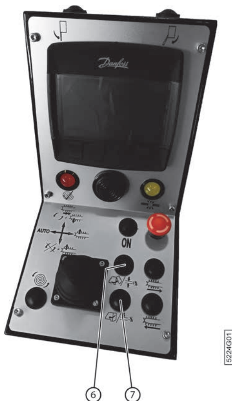
Fig. 73: Opening and/or closing the pressing chamber via the control console
