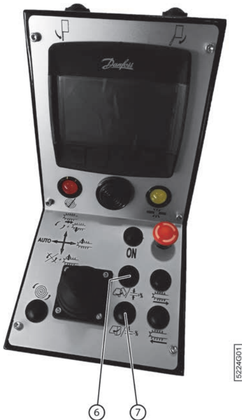
Fig. 74: Adjusting the thickness of the flax layer via the control console
