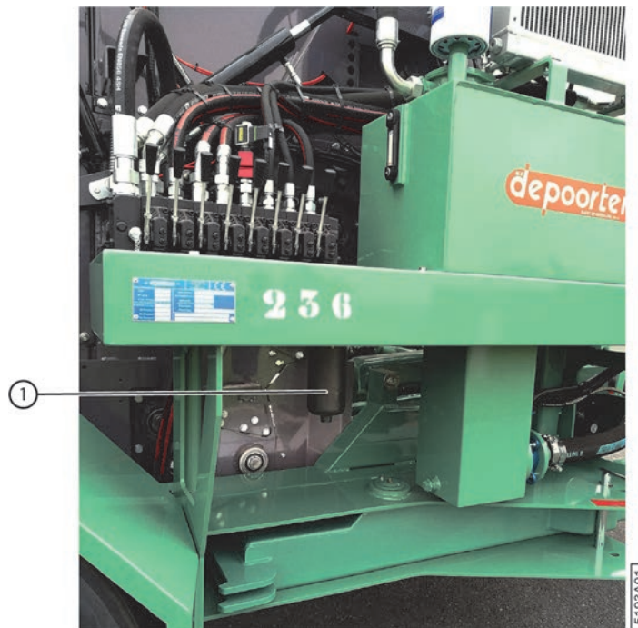
Fig. 100: Replacing the high-pressure filter
