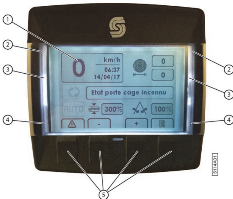
Fig. 57: The control screen
