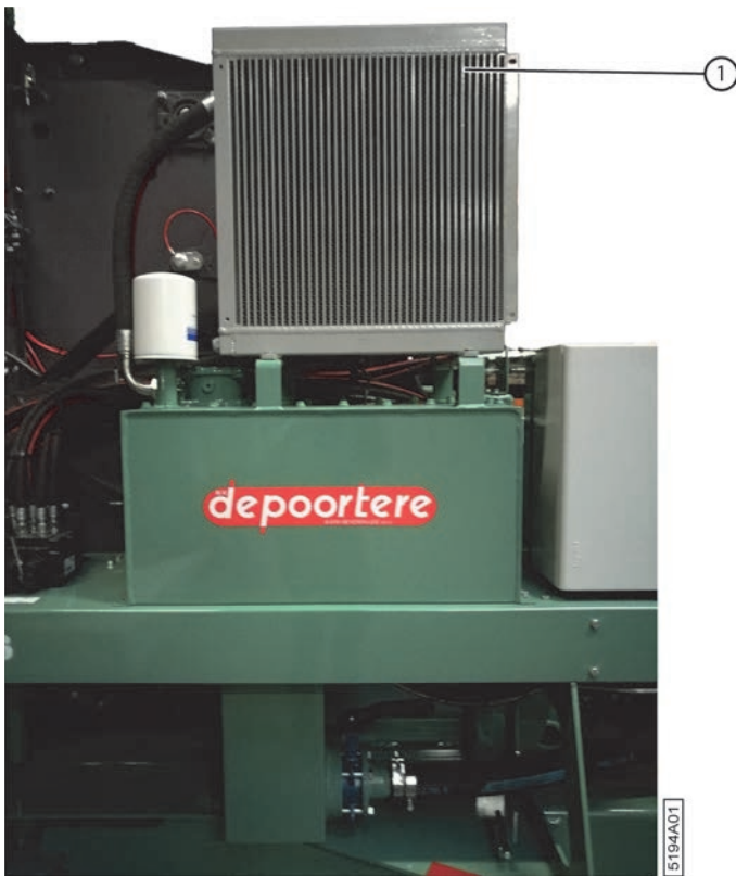
Fig. 101: Cleaning the radiator for the hydraulic oil
