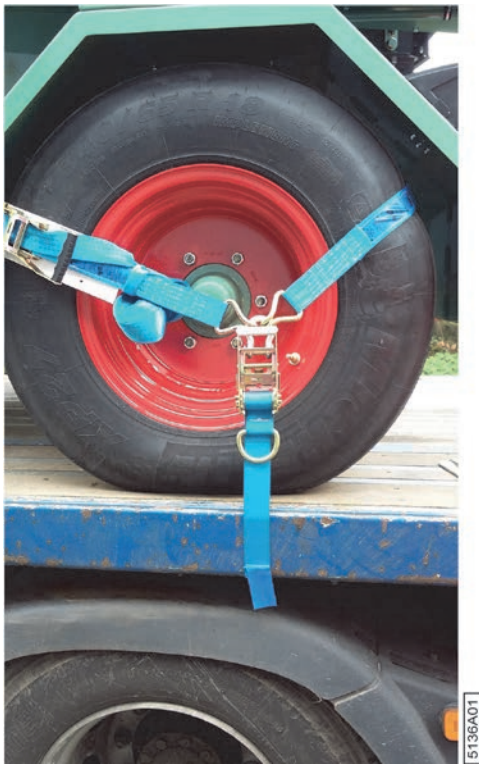
Fig. 43: Secure the tyres
