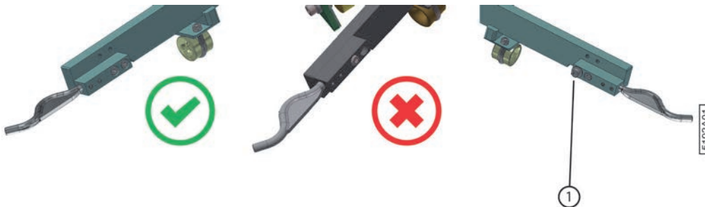
Fig. 137: Checking the position of the block of the finger
