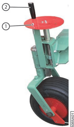
Fig. 80: Adjusting the height of the pick-up
