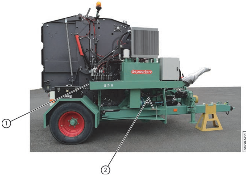
Fig. 1: Location of the identification plate and the chassis number on the machine
