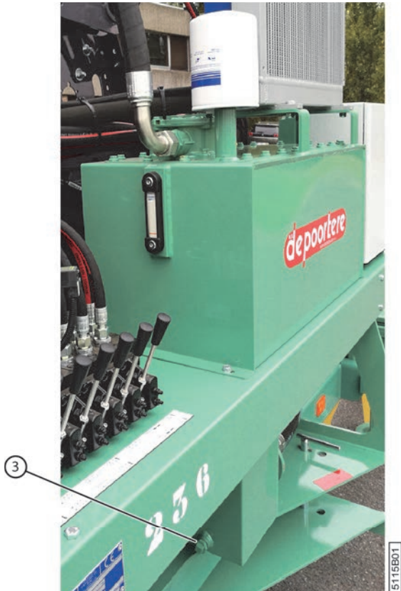
Fig. 142: Draining hydraulic tank
