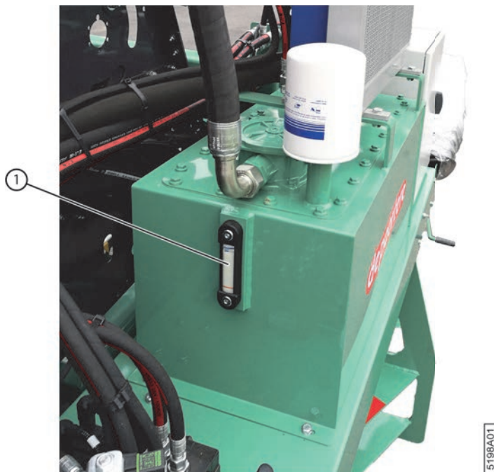
Fig. 106: Hydraulic oil level
