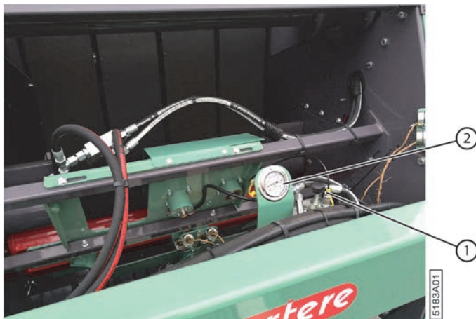
Fig. 88: Adjusting the clamping pressure in the pressing chamber
